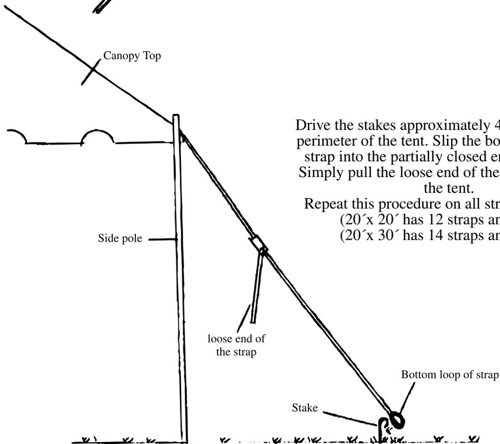
Drive the stakes approximately 4' out around the perimeter of the tent. Slip the bottom loop of the strap into the partially closed end of the stake. Simply pull the loose end of the strap to tension the tent.
