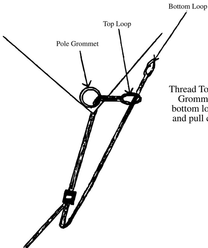
Thread Top Loop through the Pole Grommet in the tent. Take the bottom loop through the top loop and pull cinching the strap to the canopy top.
